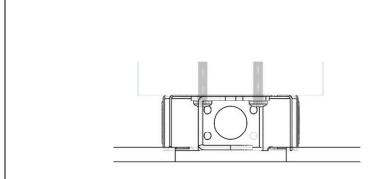
HANGER BRACKET must point in the direction of the run. This will allow for the hanger location to be modified in order to keep it plumb.
