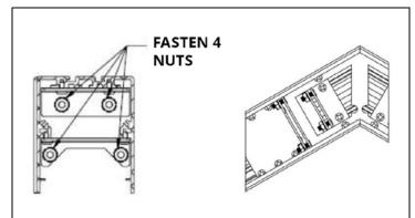
**STEP 4.** Fasten the nuts at the joining brackets to ensure a tight fit. Re-install the reflectors and the lenses.
