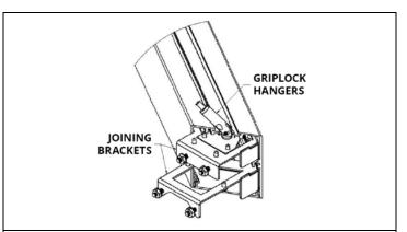
STEP 2. Install Griplocks into all six corners. Use Loctite to insure proper fastening. The Griplock must point towards the central axis of the fixture.
