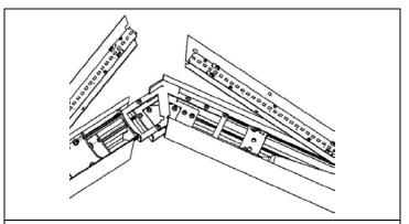
**STEP 3.** Remove lenses reflectors at the two joining sections. Join the two sections by sliding the two brackets into the adjoining section.
