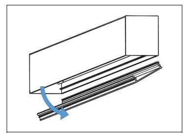
**STEP 1.** For LED board maintenance, remove lens (C) starting at one end. Pull one side first, rotate, and detach. The LED boards are now accessible
