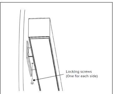
**STEP 6.** Lock fixture to wall mounts by re-attaching locking screws.
