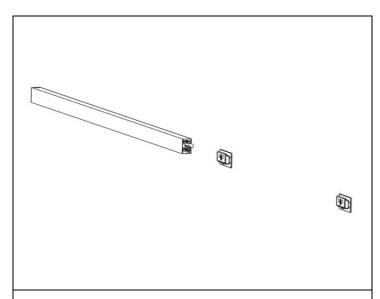
**STEP 5.** Install both wall mounting plates for the next fixture as per standard instructions.
