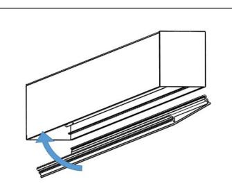
STEP 9. Perform this step only to gain access to optional emergency/battery pack. Re-attach lens. Start with one side first and close the other side starting from the corner. Make sure lens gaskets are in place and compressed between lens and fixture housing.
