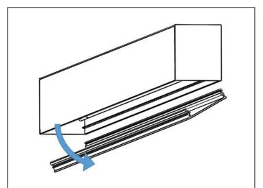
**STEP 3.** For both the start fixture and the next fixture to be joined (mid/end), remove lens starting at one end. Pull one side first, rotate and detach. Keep lens.
