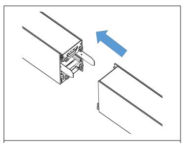
**STEP 6.** Align mid/end fixture with the start and slide into place. Secure with screws. Perform all necessary wiring between fixtures.
