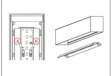
STEP 8. Perform this step only to gain access to optional emergency/battery pack. Remove reflector mounting screws and reflector/LED assembly. Note fixtures with optional emergency pack have a test switch and indicator light mounted on the reflector. Re-attach reflector with (2) mounting screws.
