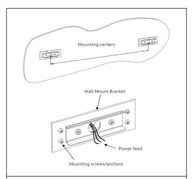
**STEP 3.** Install both wall mounting plates using (4) fasteners for each plate. Make sure the plate on wire entry side completely seals the electrical box and the two plates are installed at the same horizontal level. Route wires through the wall mount plate.
