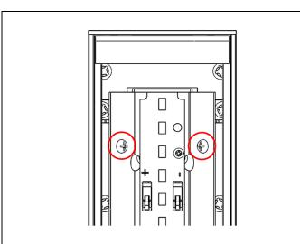
STEP 2. For driver maintenance, first unscrew the reflector assembly.
