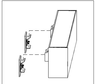
**STEP 4.** Attach luminaire to wall plates.
