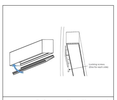
STEP 7. Re-install reflector assemblies and lenses. Finish mounting fixture with locking screws.
