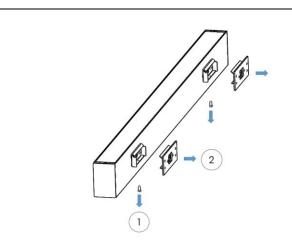
**STEP 2.** Remove the locking screws from each of the (2) wall brackets. Detach the wall mount plates (B) from the luminaire enclosure. Use mounting plate and mounting location diagram to mark location of mounting fasteners (by others).
