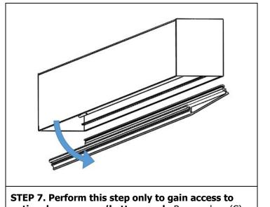
optional emergency/battery pack. Remove lens (C) starting at one end. Pull one side first, rotate and detach. Keep lens.
