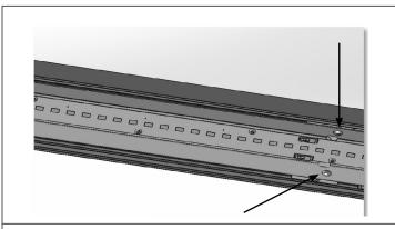
**STEP 6.** Perform this step only to gain access to fixture driver: Remove reflector mounting screws and reflector/LED assembly. Note fixtures with optional emergency pack have a test switch and indicator light mounted on the reflector.
