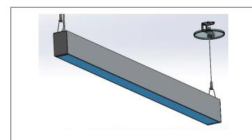
**STEP 9.** Re-attach lens. Start with one side first and close the other side starting from the corner.
