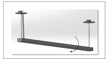
**STEP 5.** Remove lens (B) starting at one end. Pull one side first, rotate and detach. Keep lens.
