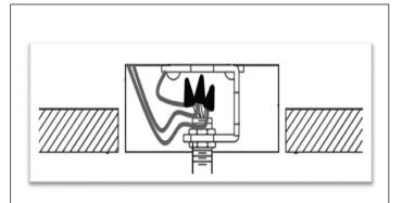
**STEP 3.** Perform electrical wiring. Optional emergency driver must be fed from the same branch circuit as the AC driver.
