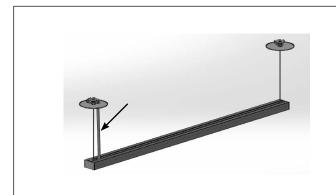
**STEP 1.** Remove fixture and hanger kit packaging; note power cord coming out at the top of the luminaire (one end only).
