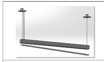
**STEP 7.** Re-attach lens. Start with one side first and close the other side starting from the corner.
