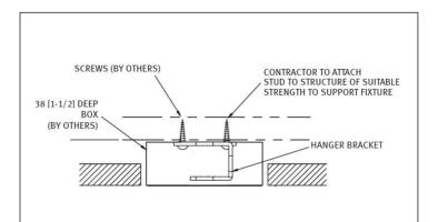
**STEP 2.** Attach both hanger brackets (F) to proper structure. One bracket needs to be attached inside electrical box with wires ready for electrical connections.
