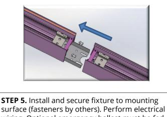
surface (fasteners by others). Perform electrical wiring. Optional emergency ballast must be fed from the same branch circuit as the AC ballast.
