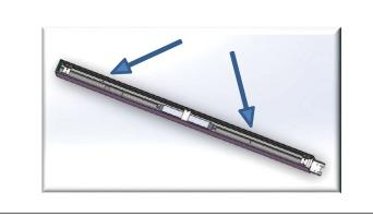
STEP 6. Re-attach reflector/LED assembly with mounting screws.
