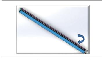
**STEP 3.** Remove lens (C) starting at one end. Pull one side first, rotate and detach. Keep lens.
