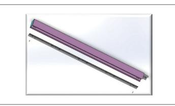
**STEP 4.** Remove reflector assembly mounting screws and reflector/LED. Note fixtures with optional emergency pack have a test switch and indicator light mounted on the reflector.
