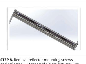
and reflector/LED assembly. Note fixtures with optional emergency pack have a test switch and indicator light mounted on the reflector.
