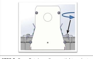
**STEP 5.** Once Retainer clips are tight against tbar fasten screws to secure Retainer Clips in location.
