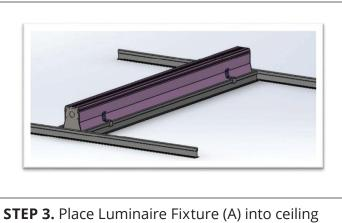
**STEP 3.** Place Luminaire Fixture (A) into ceiling and rest on tbar.
