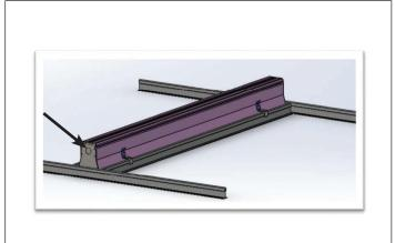
**STEP 9.** Bring electrical supply to the fixture as needed. Make sure all Retaining Clips are secured and fastened.
