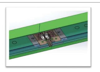
**STEP 7.** Complete luminaire attachment to wall plates and secure it in place by re-attaching (2) wall bracket mounting screws. Make sure supply wires are not pinched while performing this step. Slide extrusion aligner into joining fixture. Then place screw through lamp socket holes and tighten.
