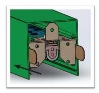
**STEP 3.** At the joiner end of the Start fixture: remove end screws. Also remove all end screws from the next fixture to be installed in the row (Middle or End luminaire) at the joining end only. Keep all parts. Slide extrusion aligners back into start fixture.
