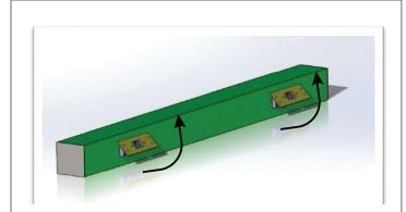
**STEP 4.** Remove (1) mounting screw from each of the (2) wall brackets on the Middle or End luminaire. Swing out wall mounting plates (B) and detach from luminaire. Keep all parts.
