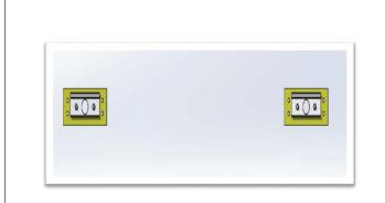
**STEP 5.** Use mounting plate and mounting location diagram to mark location of mounting fasteners (by others). Repeat for remainder of run.
