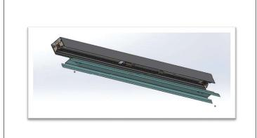
**STEP 8.** Reflector can be installed now only if access to ballast is not required. Note fixtures with optional emergency pack have a test switch and indicator light mounted on the reflector.
