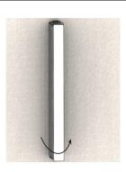
**STEP 9.** Re-attach lens. Start with one side first and close the other side starting from the corner. Make sure lens gaskets are in place and compressed between lens and fixture housing.
