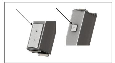
**STEP 5.** If mounting surface is uneven, apply silicone caulking on the perimeter of both back mounting gaskets (B) to ensure proper water tightness around wire entry and mounting holes.
