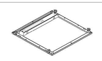
**STEP 1.** Remove fixture and all supplied parts from packaging. **DO NOT REMOVE** the protective film from the front surface of the fixture. Fixture is shipped with T-bar brackets installed.
