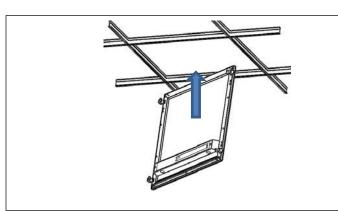
**STEP 2.** Remove ceiling tiles (where fixture is to be installed) and adjacent tiles for easy access during installation. Install fixture into T-bar grid.
