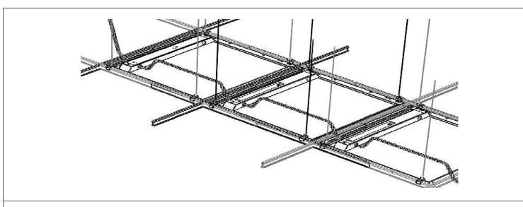
**STEP 6.** Typical daisy chained continuous rows installation, repeat steps 1-6 for all fixtures in a row. Make sure all fixtures are correctly aligned and orientated.
