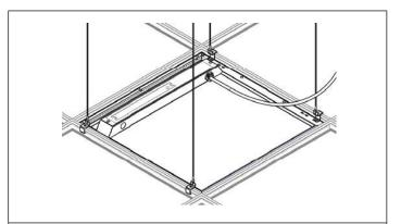
**STEP 4.** Secure fixture to structure above by attaching security wire (supplied by others) to T-bar brackets at all mounting points.
