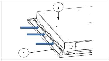
**STEP 5.** Secure the fixture to the **hanger bracket base [1]** by first inserting the tabs on the left side of the **hanger bracket [2]** into the slots of the **hanger bracket base [1]**.
