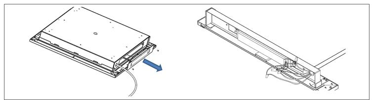
**STEP 4.** Unscrew and remove driver access panel to expose the driver. Insert line voltage through cut out and wire integral driver to line voltage. (Refer to wiring diagram from pg.2). Re-attach access panel to hanger bracket base.
