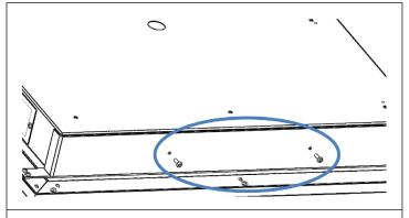
**STEP 6.** Secure luminaire to hanger bracket base using the #8 1/2" screws.
