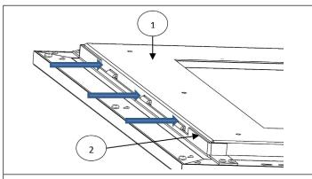
**STEP 5.** Secure the fixture to the **hanger bracket base [1]** by first inserting the tabs on the left side of the **hanger b racket [2]** into the slots of the **hanger bracket base [1]**.
