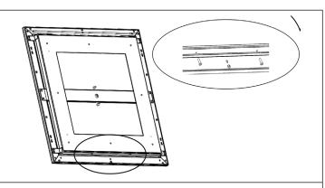
**STEP 6.** Secure lumin aire to hanger bracket base using the #8 1/2" screws.
