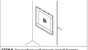
**STEP 8.** For surface wall mount, install hanger bracket base on to the wall.
