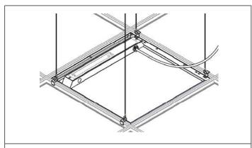
**STEP 4.** Secure fixture to structure above by attaching security wire (supplied by others) to T-bar brackets at all mounting points.
