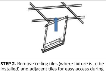
installed) and adjacent tiles for easy access during installation. Install fixture into T-bar grid.
