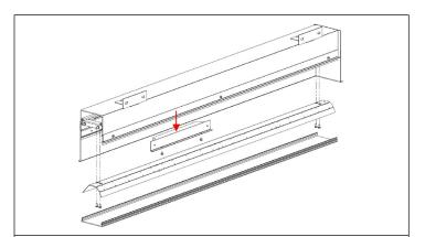
For driver maintenance, continue by removing the reflector assembly. Remove driver mounting plate assembly, and service driver as required.
