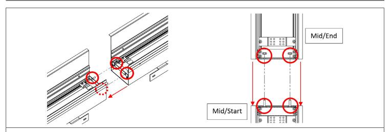
**STEP 6.** For continuous runs, with the reflector and lens removed, attach the joiner brackets of adjacent luminaires using the two screws circled. Connect wires between luminaires as per the wiring diagram.
