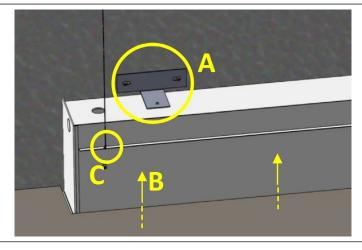
**STEP 5.** Install Wall Mounting Brackets above ceiling (A). Lift luminaire up into ceiling and reattach to Wall Mounting Bracket (B) by fastening them from the inside of the luminaire body. Secure suspension cables to holes on Fascia (C).
