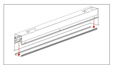
For LED board maintenance, remove the lens by gently pressing into the middle of the lens near the endcap and prying up the exposed edge.
