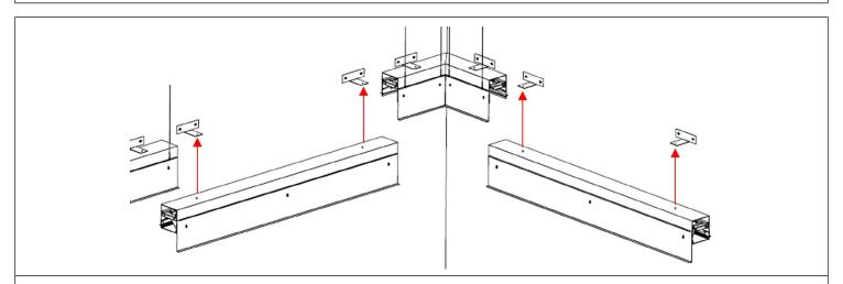
**STEP 7.** If using corners, remove lens, reflectors and wall brackets, then install them into ceiling as per step 5. It is recommended to install corners before adjacent luminaires. Join corner units with adjacent luminaire as per step 6. Reinstall lens and reflectors.
