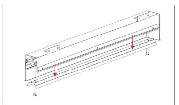
**STEP 3.** Unscrew fasteners to remove reflector assembly
