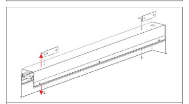
**STEP 4.** Unscrew fasteners from inside of luminaire body to free wall mounting brackets.
