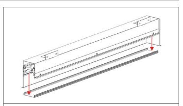
**STEP 2.** Remove the lens by gently pressing into the middle of the lens near the endcap and prying up the exposed edge.
