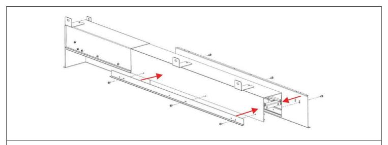
**STEP 9.** Reinstall Fascia and Wall Spacer.
