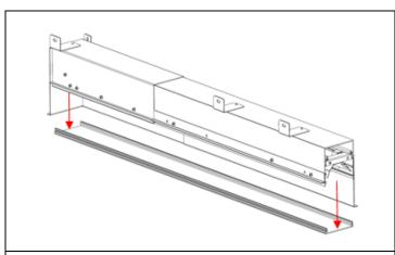
**STEP 2.** Remove the lens by gently pressing into the middle of the lens near the endcap and prying up the exposed edge.
