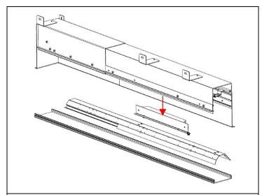
STEP 2. For driver maintenance, continue by removing the reflector assembly. Remove driver mounting plate assembly, and service driver as required.
