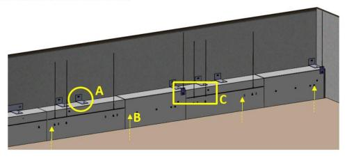
STEP 11. Install Wall Mounting Brackets above ceiling (A). Lift luminaire up into ceiling and reattach to Wall Mounting Bracket (B) by fastening them from the inside of the luminaire body. Secure suspension cables to holes on Fascia and Telescopic Suspension Hanger (C).
