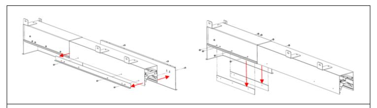
**STEP 3.** Unscrew fasteners to remove Fascia, Wall Spacer, and Spacer Plates.
