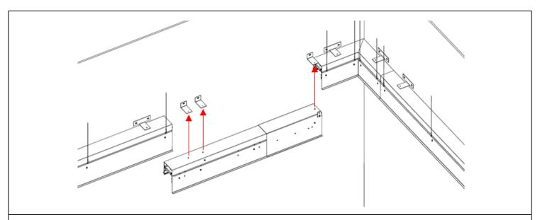
STEP 1. If corners are used, it is recommended that corner units be installed before any telescopic luminaires. Ensure the reflector and lens is removed from the corner unit. Install the telescopic luminaire as per standard instructions (Step 11).
