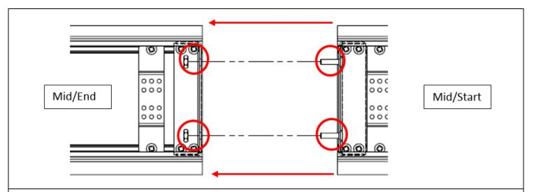
STEP 2. For continuous runs, remove the nut from the screw on the installed fixture and secure the joiner brackets of each luminaire by fastening screws through holes circled. Connect wires as described in the wiring diagram.
