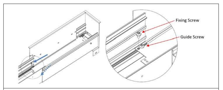
STEP 7. Remove indicated Fixing Screws on both sides of luminaire body. Ensure the Guide Screws are loose, but do not remove them.
