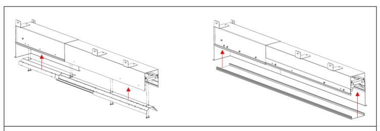
**STEP 3.** Once installation is complete, secure the reflector and lens back to the luminaire.
