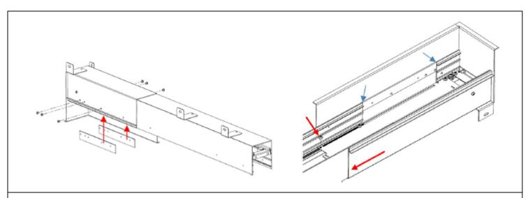
STEP 8. Install newly-cut Spacer Plates. Using the new telescopic enclosure, slide the telescopic portion over the body until gap between Spacer Plates and body is closed. Reinsert and tighten the Fixing Screws. Tighten Guide Screws. Note: Keeping the body and telescopic portion aligned while sliding will allow for smooth adjustment.
