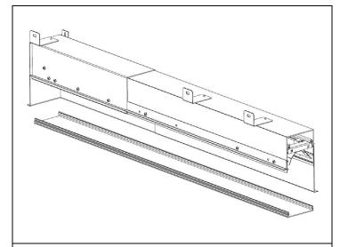
**STEP 1.** For LED board maintenance, remove the lens by gently pressing into the middle of the lens near the endcap and prying up the exposed edge. The LED boards are now accessible.
