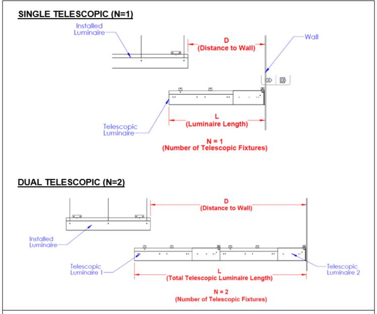
**STEP 5.** Measure the Telescopic Luminaire Length, including the length of any flanges if applicable (L). Then measure the distance from the Installed Luminaire to the Wall or next fixture (D). For arrangements requiring a single telescopic luminaire, N=1. For arrangements requiring dual telescopic luminaires, N=2.
