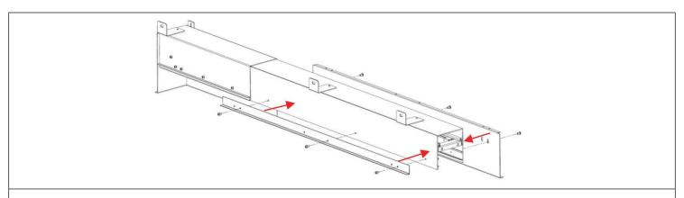
STEP 9. Reinstall Fascia and Wall Spacer.
