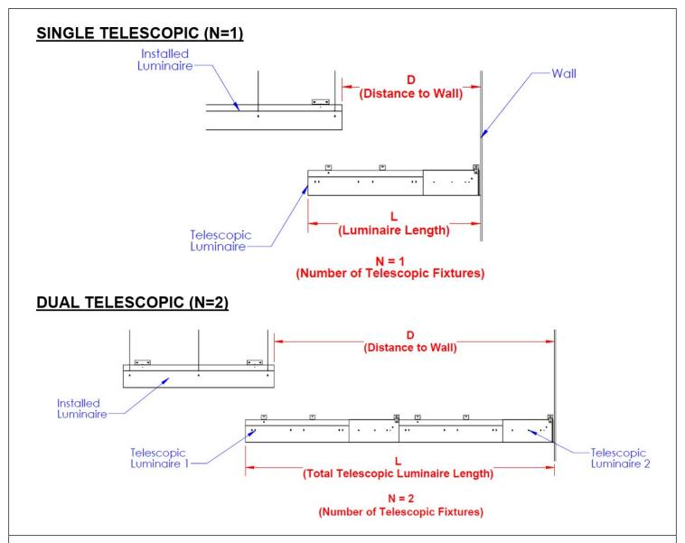
**STEP 5.** Measure the Telescopic Luminaire Length, including the length of any flanges if applicable (L). Then measure the distance from the Installed Luminaire to the Wall or next fixture (D). For arrangements requiring a single telescopic luminaire, N=1. For arrangements requiring dual telescopic luminaires, N=2.
