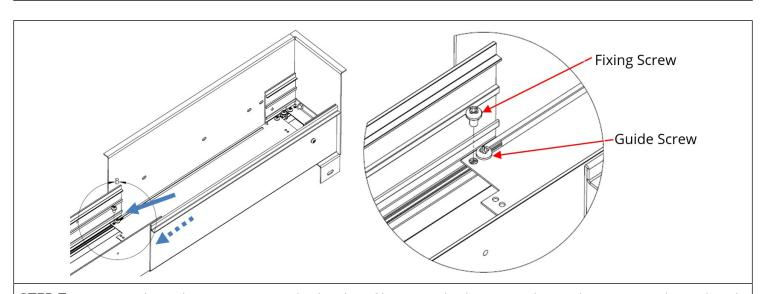
**STEP 7.** Remove indicated Fixing Screws on both sides of luminaire body. Ensure the Guide Screws are loose, but do not remove them.
