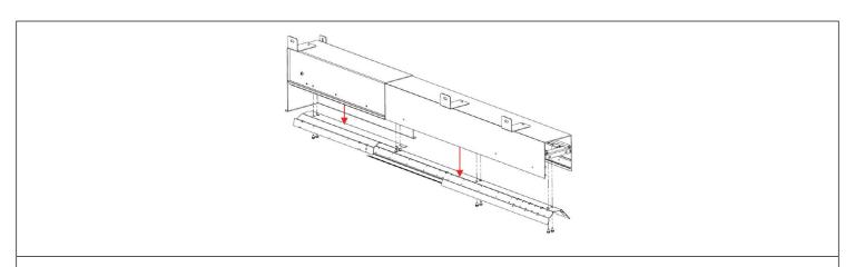
**STEP 4.** Unscrew fasteners and remove reflector assembly.
