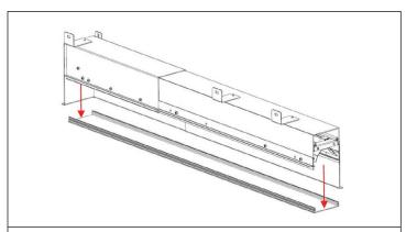
**STEP 2.** Remove the lens by gently pressing into the middle of the lens near the endcap and prying up the exposed edge.
