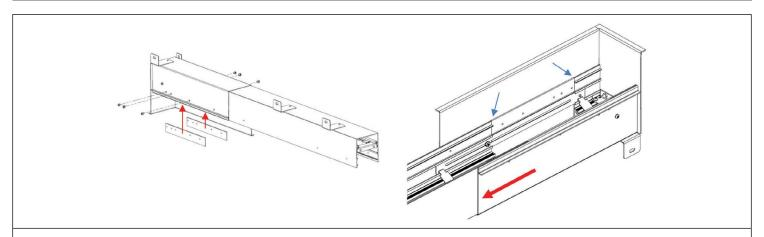
**STEP 8.** Install newly-cut Spacer Plates. Slide the telescopic portion over the body until gap between Spacer Plates and body is closed. Reinsert and tighten the Fixing Screws. Tighten Guide Screws.
