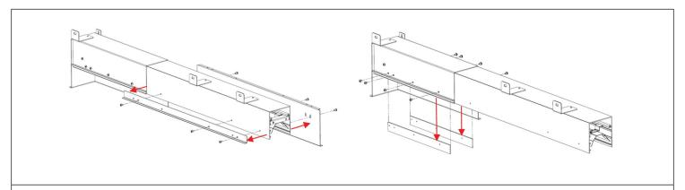
STEP 3. Unscrew fasteners to remove Fascia, Wall Spacer, and Spacer Plates.
