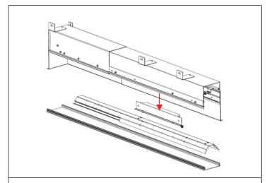
For driver maintenance, continue by removing the reflector assembly. Remove driver mounting plate assembly and service driver as required.
