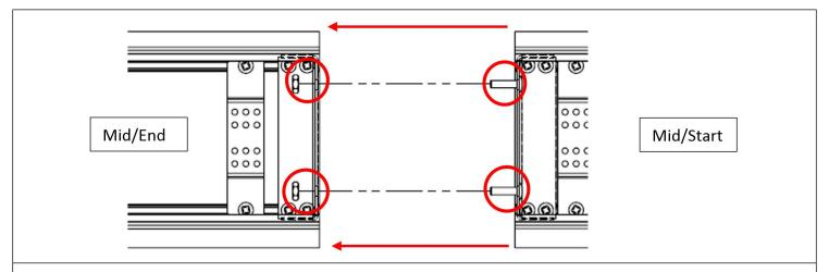
**STEP 13.** For continuous runs, remove the nut from the screw on the installed fixture and secure the joiner brackets of each luminaire by fastening screws through holes circled. Connect wires as described in the wiring diagram.
