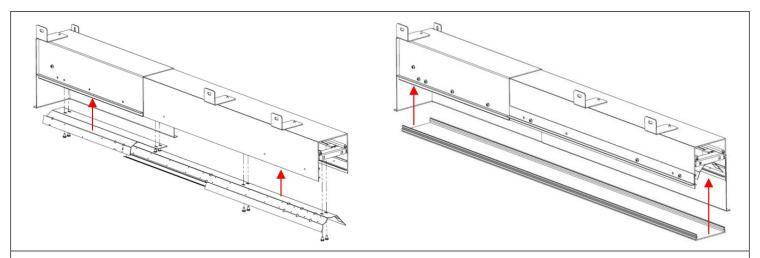
**STEP 14.** Once installation is complete, secure the reflector and lens back to the luminaire.
