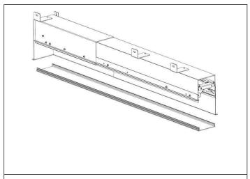
For LED board maintenance, remove the lens by gently pressing into the middle of the lens near the endcap and prying up the exposed edge.
