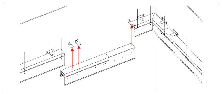
**STEP 12.** If corners are used, it is recommended that corner units be installed before any telescopic luminaires. Ensure the reflector and lens is removed from the corner unit. Install the telescopic luminaire as per Step 11.
