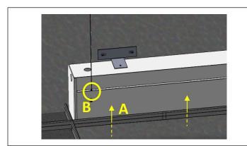
**STEP 4.** Lift luminaire up into ceiling and fasten to wall (A). Secure suspension cables to holes on fascia (B).
