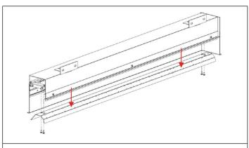
STEP 3. Unscrew fasteners to remove reflector assembly
