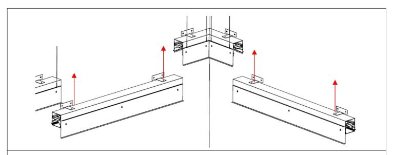
**STEP 6.** If using corners, remove lens and reflectors, then install them into ceiling as per step 4. It is recommended to install corners before adjacent luminaires. Join corner units with adjacent luminaire as per step 5. Reinstall lens and reflectors.
