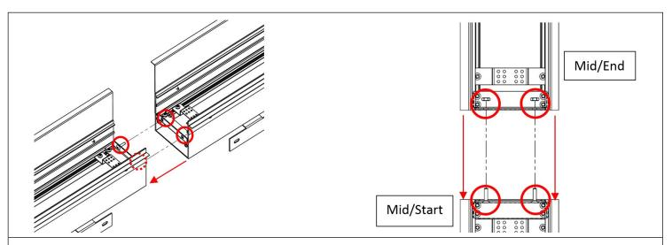
**STEP 5.** For continuous runs, with the reflector and lens removed, attach the joiner brackets of adjacent luminaires using the two screws circled. Connect wires between luminaires as per the wiring diagram.
