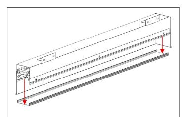
For LED board maintenance, remove the lens by gently pressing into the middle of the lens near the endcap and prying up the exposed edge.
