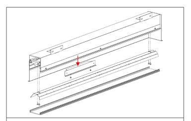
For driver maintenance, continue by removing the reflector assembly. Remove driver mounting plate assembly, and service driver as required.
