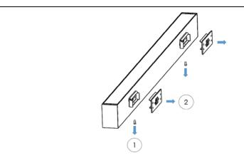
**STEP 2.** Remove the locking screws from each of the (2) wall brackets. Detach the wall mount plates (B) from the luminaire enclosure. Use mounting plate and mounting location diagram to mark location of mounting fasteners (by others).
