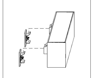
**STEP 4.** Attach luminaire to wall plates.
