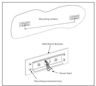
STEP 3. Install both wall mounting plates using (4) fasteners for each plate. Make sure the plate on wire entry side completely seals the electrical box and the two plates are installed at the same horizontal level. Route wires through the wall mount plate.
