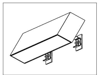
**STEP 5.** With the luminaire attached to the wall plates and rotated about 45 degrees, perform electrical wiring. Optional emergency ballast must be fed from the same branch circuit as the AC ballast.
