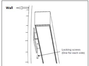
**STEP 6.** Lock fixture to wall mounts by re-attaching locking screws.
