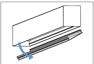
STEP 7. Perform this step only to gain access to optional emergency/battery pack. Remove lens (C) starting at one end. Pull one side first, rotate and detach. Keep lens.
