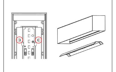
STEP 8. Perform this step only to gain access to optional emergency/battery pack. Remove reflector mounting screws and reflector/LED assembly. Note fixtures with optional emergency pack have a test switch and indicator light mounted on the reflector. Reattach reflector with (2) mounting screws.
