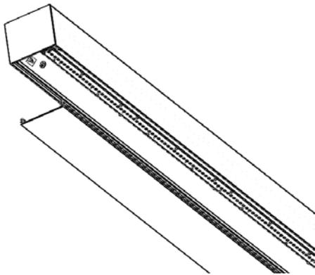
**Step 1:** For LED board and driver maintenance, remove the lens from the bottom of the unit. The LED boards are now accessible.
