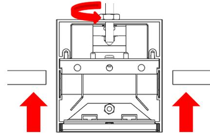
**Step 6:** Make sure to feed ready rod (by others) through mounting locations and adjust nut to ensure fixture is parallel with drywall, insert fixture all the way through the opening in the ceiling.
