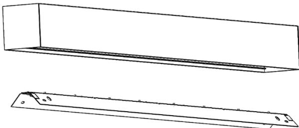
**Step 3:** Remove reflector assembly from unit.
