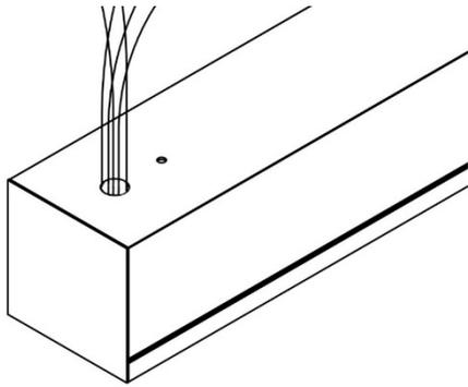
**Step 5:** Run wires through junction box and out through the hole in the top of the fixture.
