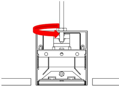
**Step 7:** Once fixture is parallel with drywall insert second nut (supplied by others) through the fixture and fasten the fixture in place. Repeat steps 6 & 7 with remaining mounting locations until fixture is parallel along entire length.
