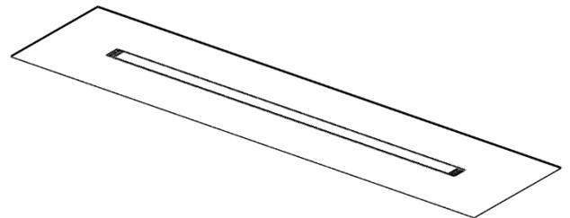
**Step 8:** Replace reflector assembly and lens.
