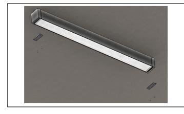
Step 9: Re-attach end plates with (4) end screws.
