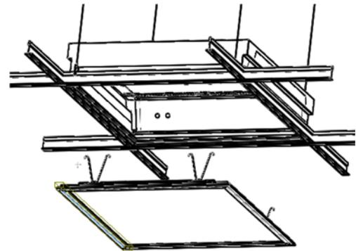
**Step 4:** Remove door from fixture. Pull door down and squeeze springs to release.
