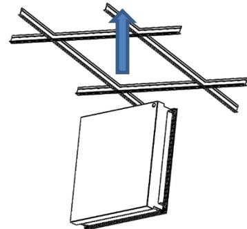
**Step 2:** Remove ceiling tiles (where fixture is to be installed) and adjacent tiles for easy access during installation. Install fixture into T-bar grid.
