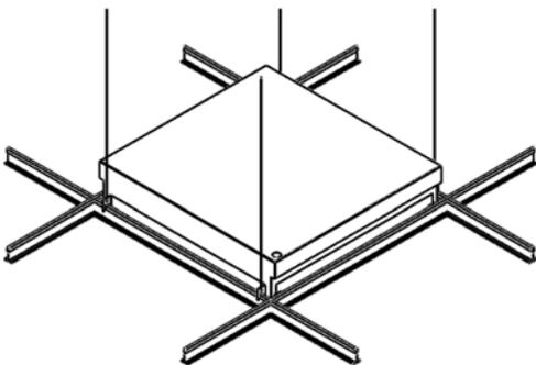
**Step 3:** Secure fixture to structure above by attaching security wire (supplied by others) to T-bar brackets at all mounting points.
