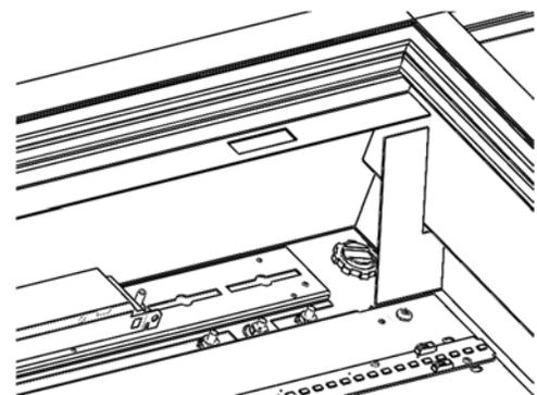
**Step 6:** Remove knock out and install the BX connector.
