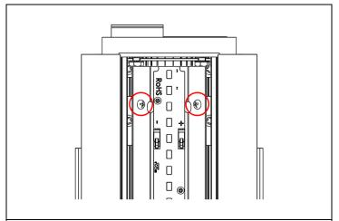
**STEP 4.** Remove reflector mounting screws.
