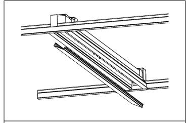
**STEP 1.** For LED board maintenance, remove the lens filler and magnet (if applicable) and remove the lens from the bottom of the unit. The LED boards are now accessible.
