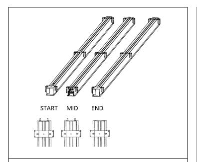
**STEP 1.** Remove fixture packaging; note marked supply wires coming out of one end of the Start luminaire and wires for row mounting connections at the opposite end.
