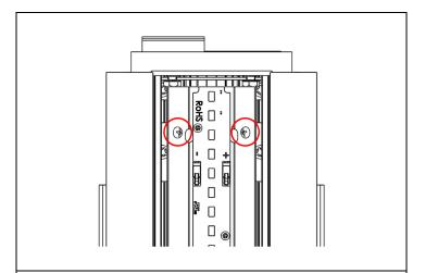
STEP 2. For driver maintenance, unscrew the reflector assembly.
