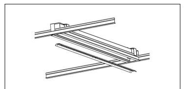
**STEP 8.** Remove reflector/LED assembly from unit. Note fixtures with optional emergency pack have a test switch and indicator light mounted on the reflector.
