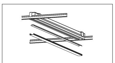
**STEP 10.** Perform electrical wiring inside the fixture. Optional emergency driver must be fed from the same branch circuit as the AC driver. Re-attach reflector/LED assembly with mounting screws.
