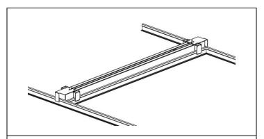
STEP 3. Place luminaire fixture (A) into ceiling and rest it onto the T-bar using the hanger bracket (B) and retainer clip.
