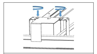
STEP 5. Once retainer clips are tight against the T-bar, fasten screws to secure retainer clips in location.
