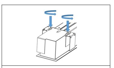
STEP 2. Ensure retainer clip (D) is loose. If not, loosen retainer clips (4).
