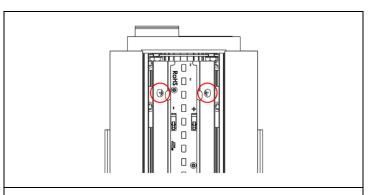
**STEP 7.** Remove reflector mounting screws.
