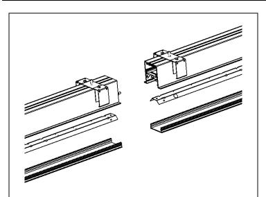
**STEP 5.** Remove reflector and LED assembly on joining ends to access the joining brackets.
