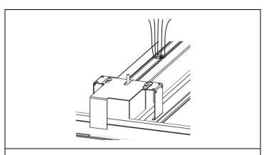
**STEP 9.** Bring electrical supply to the fixture as needed. Make sure all retaining clips are secured and fastened.
