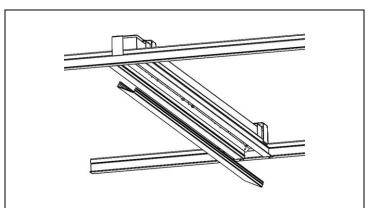
STEP 6. Remove lens (E) starting at one end. Pull one side first, rotate and detach. Keep lens.
