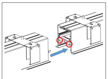
**STEP 6.** Align mid/end fixture and slide it into place. Secure with joining hardware. Reinstall reflector/LED assembly and lens in both fixtures. Perform necessary wiring between fixtures. Repeat steps for remaining fixtures.
