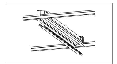
STEP 11. Re-attach lens. Start with one side first and close the other side starting from the corner.
