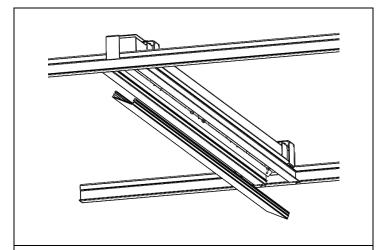
**STEP 3.** Remove lens starting at one end. Pull one side first, rotate and detach. Keep lens.
