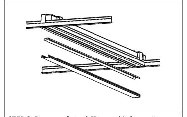
**STEP 3.** Remove reflector/LED assembly from unit.
