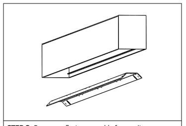
**STEP 3.** Remove reflector assembly from unit.
