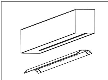
**STEP 4.** For both the start fixture and the next fixture to be joined (mid/end), remove reflector mounting screws and reflector/LED assembly. Note fixtures with optional emergency pack have a test switch and indicator light mounted on the reflector.
