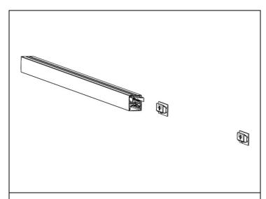
**STEP 5.** Install both wall mounting plates for the next fixture as per standard instructions.
