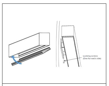
STEP 7. Re-install reflector assemblies and lenses. Finish mounting fixture with locking screws.
