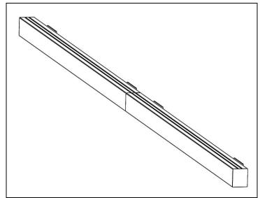
STEP 8. Joined luminaires. Complete remaining fixtures installation as needed.
