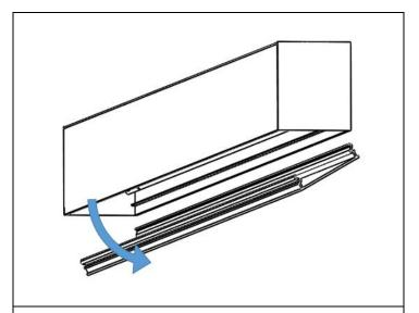
**STEP 1.** For LED board maintenance, remove lens (C) starting at one end. Pull one side first, rotate, and detach. The LED boards are now accessible
