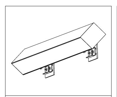
**STEP 5.** With the luminaire attached to the wall plates and rotated about 45 degrees, perform electrical wiring. Optional emergency ballast must be fed from the same branch circuit as the AC ballast.
