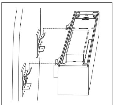
**STEP 4.** Attach luminaire to wall plates.
