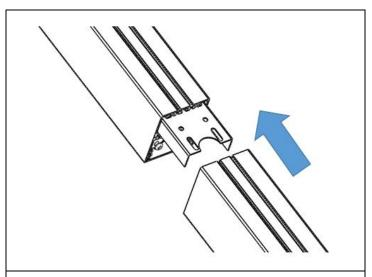
**STEP 6.** Align mid/end fixture with the start and slide into place. Secure with screws. Perform all necessary wiring between fixtures.
