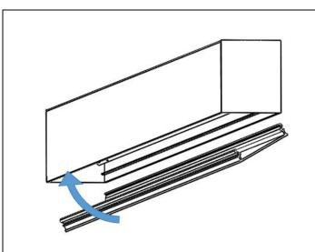
STEP 9. Perform this step only to gain access to optional emergency/battery pack. Re-attach lens. Start with one side first and close the other side starting from the corner. Make sure lens gaskets are in place and compressed between lens and fixture housing.
