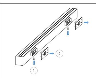
**STEP 2.** Remove the locking screws from each of the (2) wall brackets. Detach the wall mount plates (B) from the luminaire enclosure. Use mounting plate and mounting location diagram to mark location of mounting fasteners (by others).
