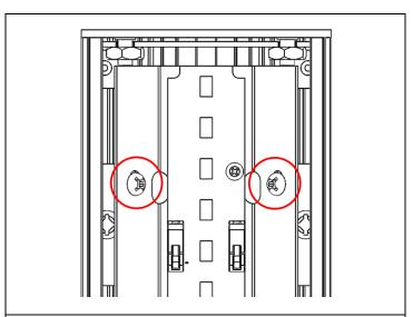
**STEP 2.** For driver maintenance, first unscrew the reflector assembly.
