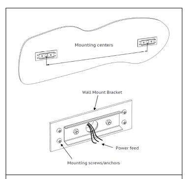
**STEP 3.** Install both wall mounting plates using (4) fasteners for each plate, making sure the two plates are installed at the same horizontal level. Route wires through the wall mount plate.
