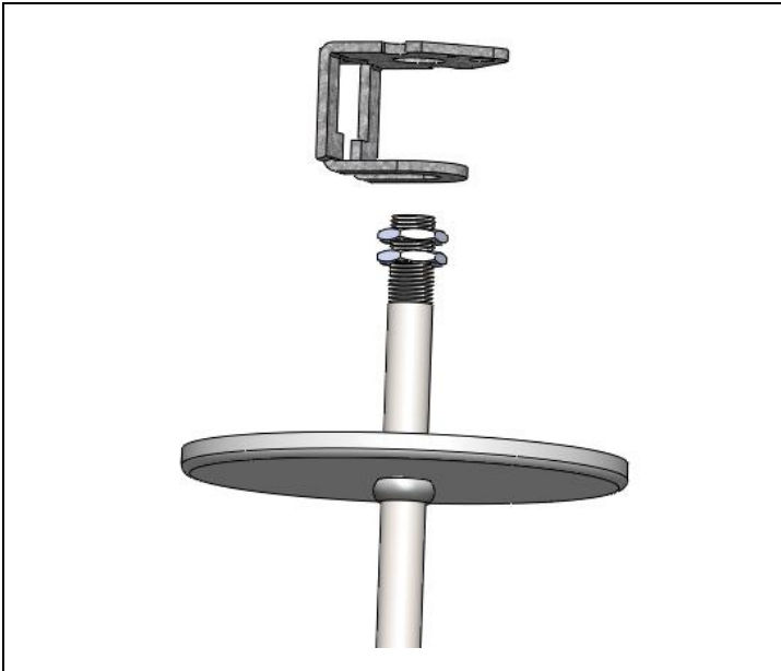
STEP 5. Attach both stems to hanger brackets.
