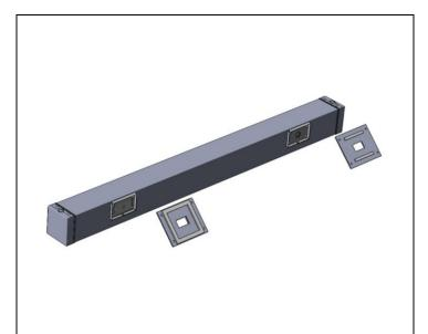
STEP 3. Detach plates from luminaire enclosure (A). Note wall mounting plate on wire entry side is fully gasketed. Use mounting plate and mounting location diagram to mark location of mounting fasteners (by others).
