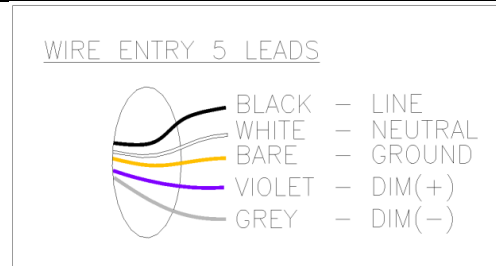
DRIVER TO LINE VOLTAGE
