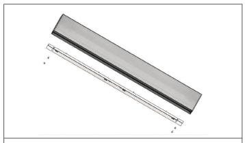
**STEP 5.** Re-attach reflector/LED assembly with mounting screws.
