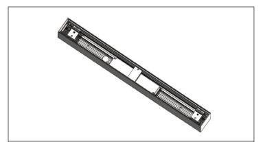
**STEP 4.** Install and secure fixture to mounting surface (fasteners by others). Perform electrical wiring. Optional emergency ballast must be fed from the same branch circuit as the AC ballast.
