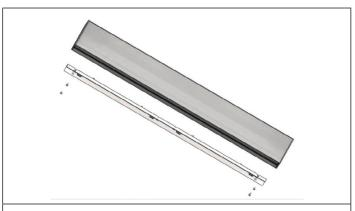
**STEP 3.** Remove reflector assembly mounting screws and reflector/LED. Note fixtures with optional emergency pack have a test switch and indicator light mounted on the reflector.
