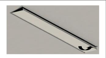
**STEP 7.** Re-attach lens. Start with one side first and close the other side starting from the corner.
