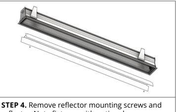
reflector. Note fixtures with optional emergency pack have a test switch and indicator light mounted on the reflector.
