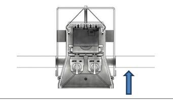
**STEP 5.** Bring electrical supply to the fixture as needed. Make sure all mounting brackets (B) are parallel to the luminaire enclosure (A) and insert fixture all the way through the opening in the ceiling.
