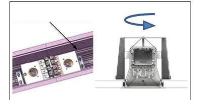
**STEP 8.** Begin tightening the mounting screws. Mounting brackets will swing out and retain the luminaire in place. Continue to tighten the screws until the luminaire flanges are flush with the ceiling.
