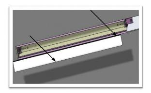
**STEP 3.** Remove lens starting at one end. Pull one side first, rotate and detach. Then remove plug at joining end of reflector to access joining kit.
