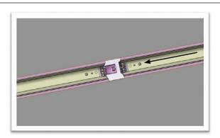
**STEP 4.** Remove lens and reflector plug on mid fixture. Then slide mid fixture; butt up to start fixture then fasten screw to wedge joiner kit.
