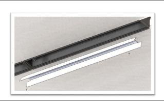
**STEP 9.** Perform electrical wiring inside the fixture and re-attach reflector with (2) mounting screws. Optional emergency ballast must be fed from the same branch circuit as the AC ballast.
