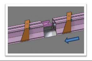
**STEP 7.** Route electrical supply from Start fixture through to mid/end fixture. Insert fixture completely through the ceiling opening and join luminaires together.
