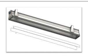
**STEP 5.** Remove reflector mounting screws and reflector. Note fixtures with optional emergency pack have a test switch and indicator light mounted on the reflector.
