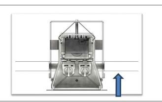
**STEP 6.** Make sure all mounting brackets (B) are parallel to the luminaire enclosure (A) and insert fixture through the opening in the ceiling. Bring fixture close to the Start fixture (already installed).
