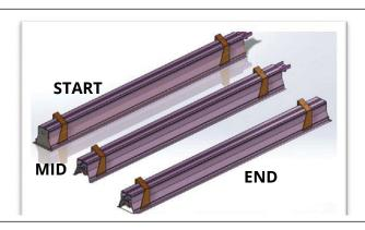
**STEP 1.** Remove fixture packaging; note marked supply wires coming out at one end of the Start luminaire and wires for row mounting connections at the opposite end.
