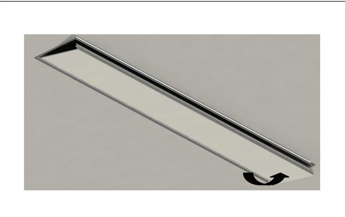
**STEP 8.** Re-attach lens. Start with one side first and close the other side starting from the corner.
