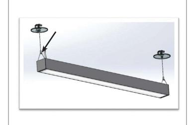
**STEP 4.** Assemble hanger kit from IS-0713A and attach (J) AC Griplok to (E) Cable w/ Crimp. Level out fixture using (J) AC Griplok.
