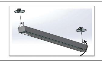
**STEP 9.** Re-attach lens. Start with one side first and close the other side starting from the corner.
