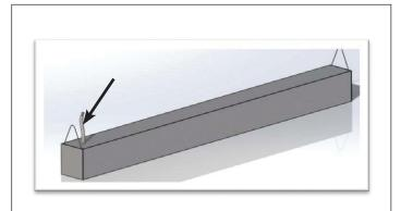
**STEP 1.** Remove fixture and hanger kit packaging; note power cord coming out at the top of the luminaire (one end only).
