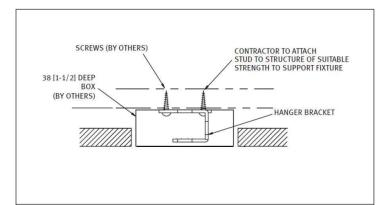
**STEP 2.** Attach both hanger brackets (H) to proper structure. One bracket needs to be attached inside electrical box with wires ready for electrical connections.
