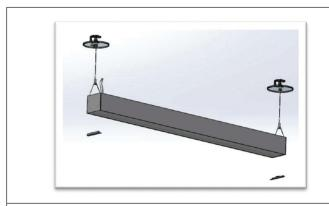
**STEP 5.** Remove filler & magnet (D). Keep all parts.
