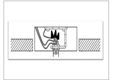
**STEP 3.** Perform electrical wiring. Optional emergency ballast must be fed from the same branch circuit as the AC ballast.
