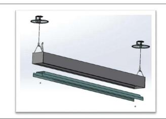
**STEP 7.** Perform this step only to gain access to fixture ballast: Remove reflector mounting screws and reflector. Note fixtures with optional emergency pack have a test switch and indicator light mounted on the reflector.
