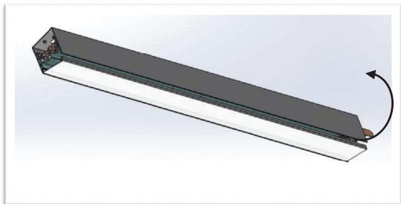
**STEP 9.** Re-attach lens. Start with one side first and close the other side starting from the corner.
