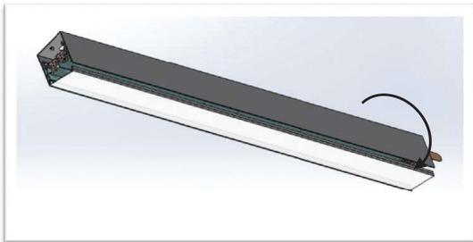
**STEP 3.** Remove lens (C) from Middle or End luminaire. Starting at one end; pull one side first, rotate and detach. Keep lens.
