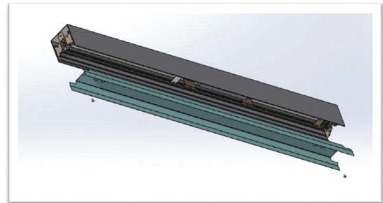
**STEP 4.** Remove reflector mounting screws and reflector. Note fixtures with optional emergency pack have a test switch and indicator light mounted on the reflector.
