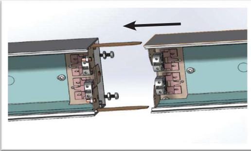
**STEP 5.** Bring fixture with the wire entry end close to the Start fixture joiner end. Attach Middle or End fixture to the Start fixture joiner end by inserting aligners from start fixture into mid/end; Make electrical connection between fixtures; place screw thru lamp socket holes and tightening with nuts to join up fixtures. Perform wiring at switch box.
