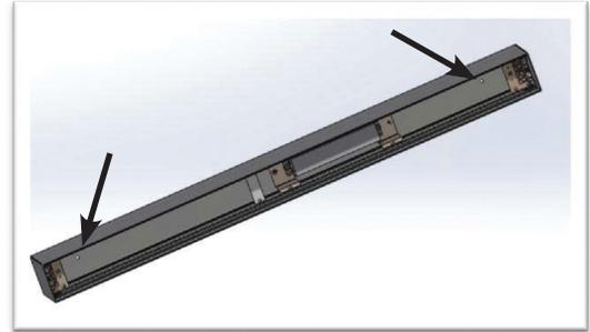
**STEP 6.** Install and secure fixture to the mounting surface (fasteners by others).
