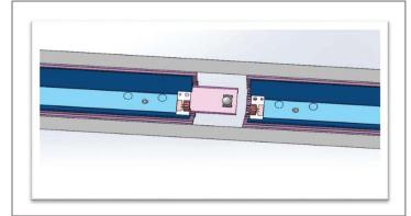
**STEP 4.** Remove lens and reflector plug on mid fixture. Make all necessary electrical connections from start fixture through mid/end fixtures. Then slide mid fixture; butt up to start fixture then fasten screw to wedge joiner kit. Repeat for remainder of run.
