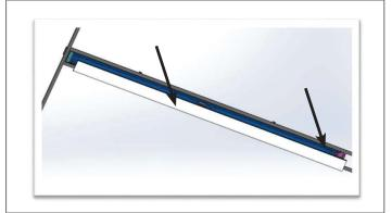
**STEP 3.** Remove lens starting at one end. Pull one side first, rotate and detach. Then remove plug at joining end of reflector to access joining kit.
