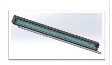
**STEP 9.** Reflector can be removed now only if access to ballast is required. Note fixtures with optional emergency pack have a test switch and indicator light mounted on the reflector. Reattach reflector (if applicable). Install lamp(s).
