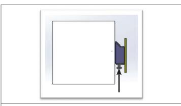
**STEP 6.** Complete luminaire attachment and secure it in place by re-attaching (2) wall bracket mounting screws. Make sure supply wires are not pinched while performing this step.
