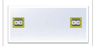
**STEP 4.** Install both wall mounting plates. Use (4) fasteners for each plate. Make sure the plate on wire entry side completely seals the electrical box and the two plates are installed at the same horizontal level. Route wires through wall mount bracket.
