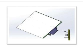
**STEP 5.** Route wires through wire entry hole to inside of fixture. Attach luminaire to wall plates.
