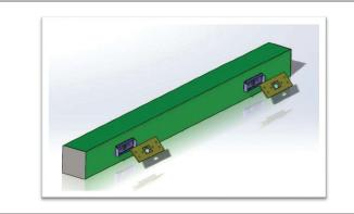
**STEP 3.** Detach plates from luminaire enclosure (A). Use mounting plate and mounting location diagram to mark location of mounting fasteners (by others).
