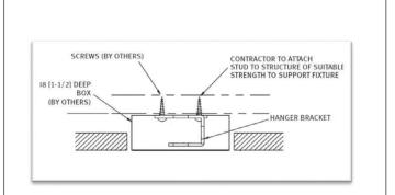
**STEP 7.** Repeat Step 4 and install Hanger bracket (1) for Mid/End Fixture. (Repeat for entire run)
