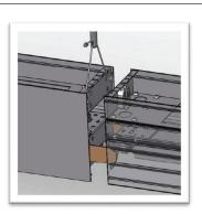
**STEP 6.** Bring fixture with the wire entry end close to the Start fixture joiner end. Attach Middle or End fixture to the Start fixture joiner end by inserting aligners from start fixture into mid/end; placing screw thru lamp socket holes and tightening with nuts to join up fixtures.
