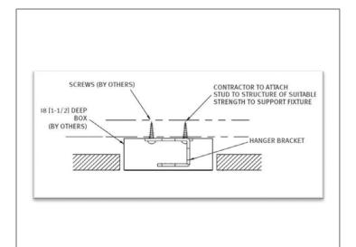
**STEP 4.** Attach hanger bracket (H) to proper mid/ end fixture. One bracket needs to be attached inside electrical box.
