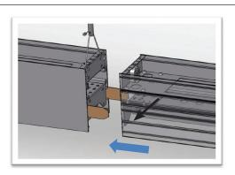
**STEP 5.** Bring Middle or End fixture with the wire end close to the Start fixture joiner end. Route wires from Start fixture through Middle/ End fixture.
