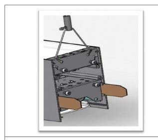
**STEP 3.** At the joiner end of the Start fixture: remove end screws (keep aligner plates inserted. Keep all parts.
