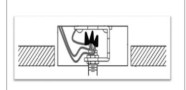
**STEP 8.** Perform electrical wiring. Optional emergency ballast must be fed from the same branch circuit as the AC ballast.
