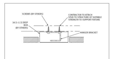
**STEP 2.** Attach both hanger brackets (G) to proper structure. One bracket needs to be attached inside electrical box with wires ready for electrical connections.
