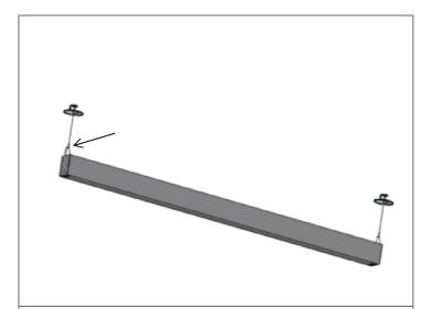
**STEP 4.** Assemble hanger kit from IS-0713A and attach (I) AC Griplok to (D) Cable w/ Crimp. Level out fixture using (I) AC Griplok.
