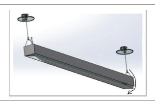
**STEP 5.** Remove lens (B) starting at one end. Pull one side first, rotate and detach. Keep lens. Follow same instructions for indirect lens.
