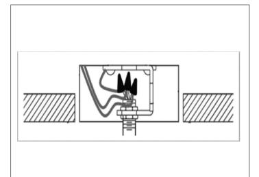
**STEP 3.** Perform electrical wiring. Optional emergency ballast must be fed from the same branch circuit as the AC ballast.
