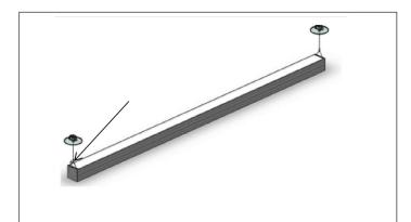
**STEP 1.** Remove fixture and hanger kit packaging; note power cord coming out at the top of the luminaire (one end only).
