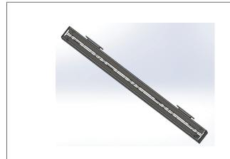
**STEP 8.** Reflector/LED assembly can be removed now only if access to driver is required. Note fixtures with optional emergency pack have a test switch and indicator light mounted on the reflector. Re-attach reflector/LED assembly (if applicable).
