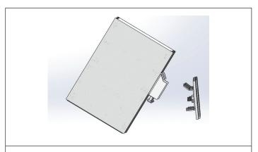
**STEP 5.** Route wires through wire entry hole to inside of fixture. Attach luminaire to wall plates.
