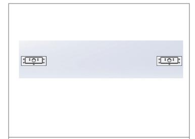
**STEP 4.** Install both wall mounting plates. Use (4) fasteners for each plate. Make sure the plate on wire entry side completely seals the electrical box and the two plates are installed at the same horizontal level. Route wires through wall mount bracket.
