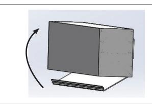
**STEP 9.** Re-attach lens. Start with one side first and close the other side starting from the corner.
