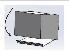
**STEP 7.** Remove lens (D) starting at one end. Pull one side first, rotate and detach. Keep lens. Follow same instructions for indirect lens.
