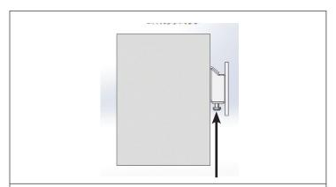
**STEP 6.** Complete luminaire attachment and secure it in place by re-attaching (2) wall bracket mounting screws. Make sure supply wires are not pinched while performing this step.
