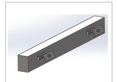
**STEP 3.** Detach plates from luminaire enclosure (A). Use mounting plate and mounting location diagram to mark location of mounting fasteners (by others).
