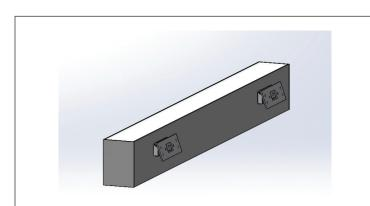
**STEP 2.** Remove (1) mounting screw from each of the (2) wall brackets. Swing out wall mounting plates (B).
