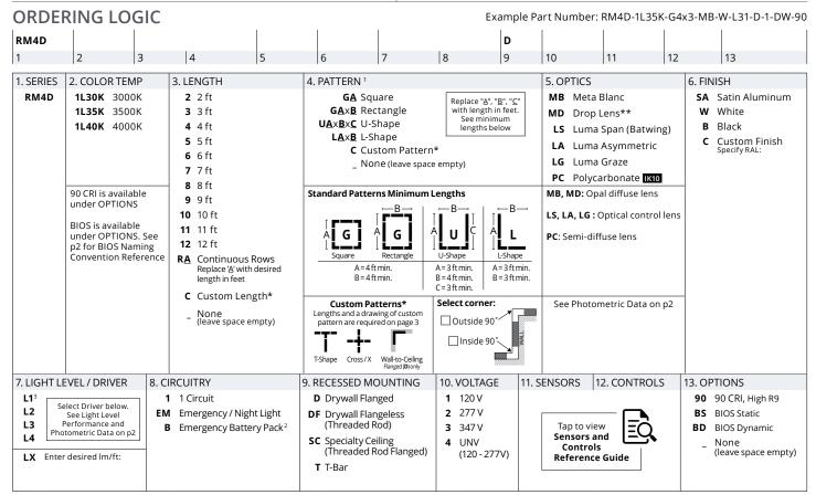
\*Consult factory. | \*\*Drop lens is not available with patterns. | 1 Pattern approval drawings showing mounting locations will be sent out upon order. | 2 Battery operates 4ft sections only. | 3 Not available with BIOS.
