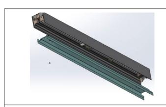
**STEP 6.** Re-attach reflector with (2) mounting screws.
