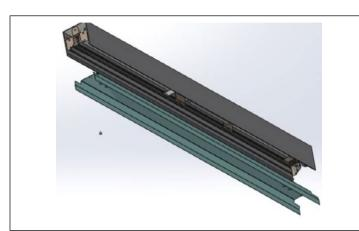
**STEP 4.** Remove reflector mounting screws and reflector. Note fixtures with optional emergency pack have a test switch and indicator light mounted on the reflector.
