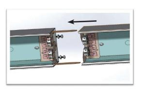
**STEP 5.** Bring fixture with the wire entry end close to the Start fixture joiner end. Attach Middle or End fixture to the Start fixture joiner end by inserting aligners from start fixture into mid/end; Make electrical connection between fixtures; place screw thru lamp socket holes and tightening with nuts to join up fixtures. Perform wiring at switch box.
