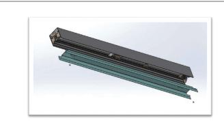
**STEP 4.** Remove reflector mounting screws and reflector. Note fixtures with optional emergency pack have a test switch and indicator light mounted on the reflector.
