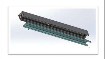
**STEP 7.** Re-attach reflector with (2) mounting screws.
