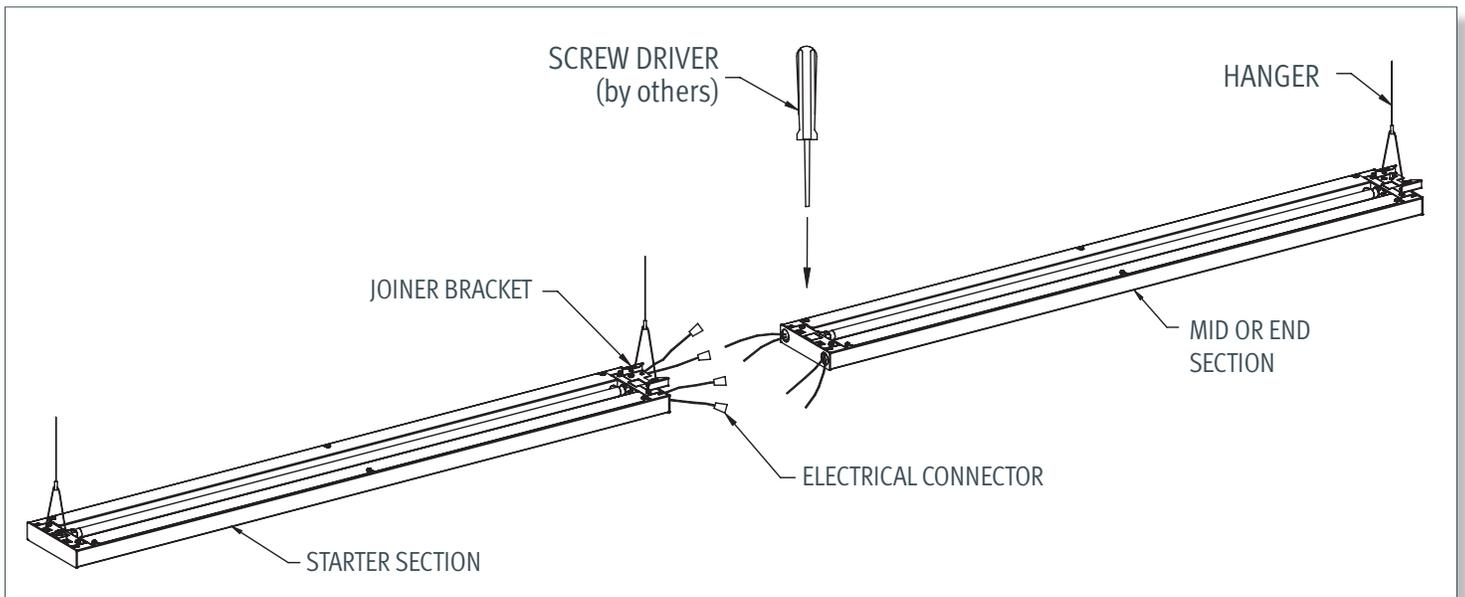
**STEP 1** Install JOINER BRACKET to the Joiner End of the START or MID SECTION.
