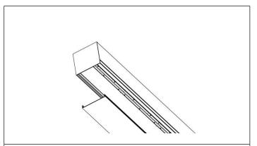
STEP 1. For LED board maintenance, remove the lens from the bottom of the unit.
