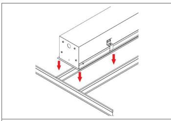
**STEP 7.** Raise fixture above the ceiling and lower the fixture onto the T-bars.
