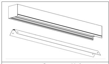
STEP 3. Remove reflector assembly from unit.
