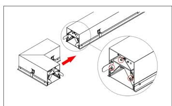
**STEP 11.** For corners, remove the lens and reflector pairs from the corner unit (see steps 2-4). Attach the corner to the preceding unit joiner brackets using 3 screws.
