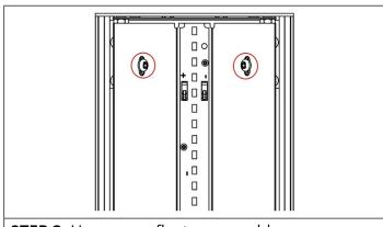
STEP 3. Unscrew reflector assembly.
