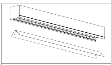
**STEP 4.** Remove reflector assembly.
