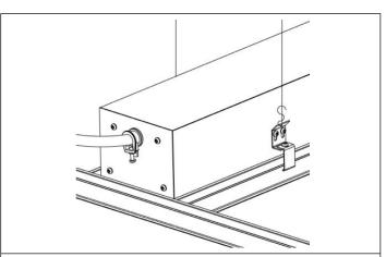
**STEP 14.** Attach safety wires to each mounting bracket. Connect cables from BX cable to the fixture driver cables. Install all ceiling tiles.
