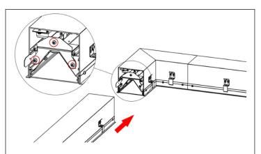
**STEP 12.** Attach the next mid/end unit to the corner unit as per step 10. Connect wires between fixtures as per the wiring diagram. Reinstall the reflector and lens in corner.
