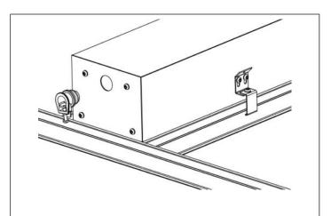
STEP 9. Knock out and install BX connector (Supplied by others). Feed BX cable (supplied by others) through connector and end plate. Tighten BX connector screw cable to wire entry plate. Reinstall reflector and lens. Skip to step 14 for stand-alone fixtures. For a grid, feed cable through the hole in the provided wire entry corner piece.
