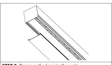
STEP 2. Remove the lens in the unit.
