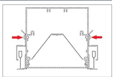
**STEP 8.** Adjust the T-bar mounting brackets snug to the T-bar frame and secure into position using the Phillips screws on the sides of the fixture.
