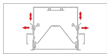
**STEP 6.** Open T-bar mounting brackets by loosening the Phillips head screws on the side of the fixture. Open the brackets to the widest position.
