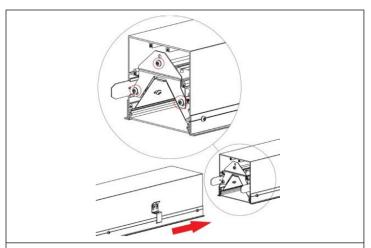
**STEP 10.** For continuous runs, remove the lens and reflector from the mid/end unit (see steps 2-4). Attach the joiner brackets of each unit using 3 screws. Reinstall the reflector and lens in mid/end.
