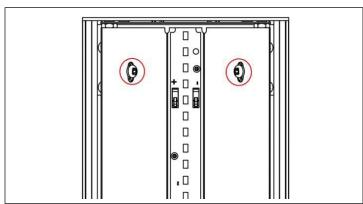
STEP 2. For driver maintenance, first unscrew the reflector assembly.
