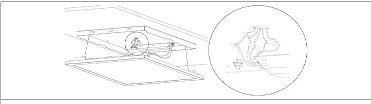
**STEP 4.** Wire integral driver to line voltage. (Refer to wiring diagram from pg.2)
