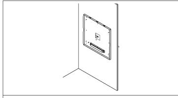
**STEP 8.** For surface wall mount, install hanger bracket base on to the wall.
