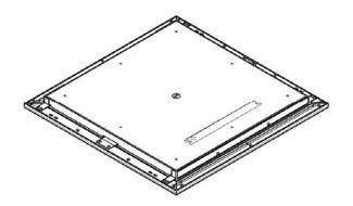
**STEP 1.** Remove fixture and all supplied parts from packaging. DO NOT REMOVE the protective film from the front surface of the fixture.
