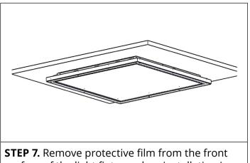
**STEP 7.** Remove protective film from the front surface of the light fixture when installation is completed.
