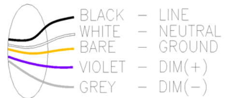
REMOTE DRIVER BOX TO LINE VOLTAGE
