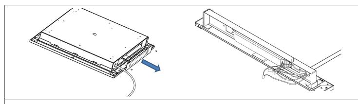
**STEP 4.** Unscrew and remove driver access panel to expose the driver. Insert line voltage through cut out and wire integral driver to line voltage. (Refer to wiring diagram from pg.2). Re-attach access panel to hanger bracket base.
