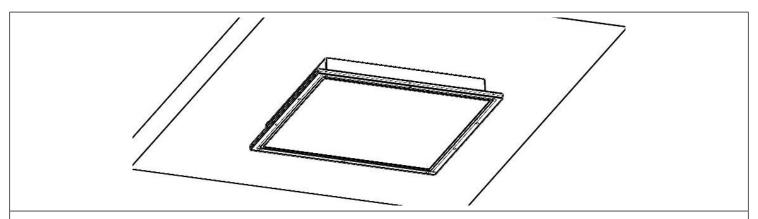
**STEP 7.** Remove protective film from the front surface of the light fixture when installation is completed.
