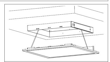
**STEP 3.** Attach safety cable from fixture to hanger bracket
