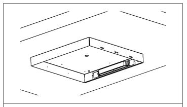
**STEP 2.** Install hanger bracket base (A) into ceiling.
