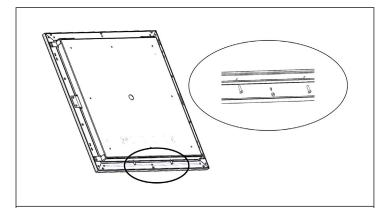
**STEP 6.** Secure luminaire to hanger bracket base using the #8 1/2" screws.
