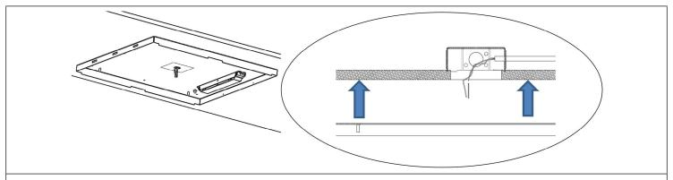
STEP 2. Install hanger bracket base (A) into ceiling.
