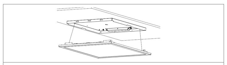
STEP 3. Attach safety cable from fixture to hanger bracket
