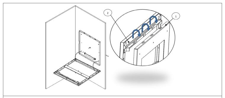
**STEP 9.** Reposition and attach safety cables to bottom of hanger bracket base and connect to luminaire. Secure the fixture to the **hanger bracket base [1]** by first inserting the tabs on the left side of the **hanger bracket [2]** into the slots of the hanger
