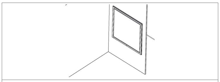
**STEP 12.** Remove protective film from the front surface of the light fixture when installation is completed.
