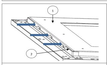
**STEP 5.** Secure the fixture to the **hanger bracket base [1]** by first inserting the tabs on the left side of the **hanger bracket [2]** into the slots of the **hanger bracket base [1]**.
