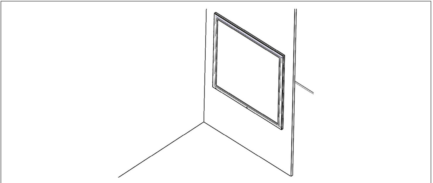
**STEP 12.** Remove protective film from the front surface of the light fixture when installation is completed.
