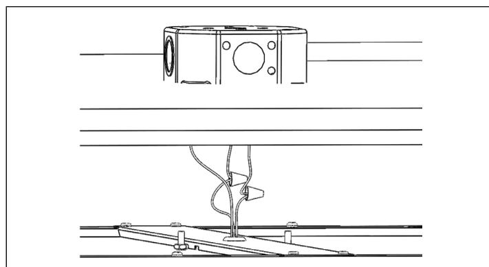
**STEP 4.** Wire fixture to remote driver. (Refer to wiring diagram from pg.2)
