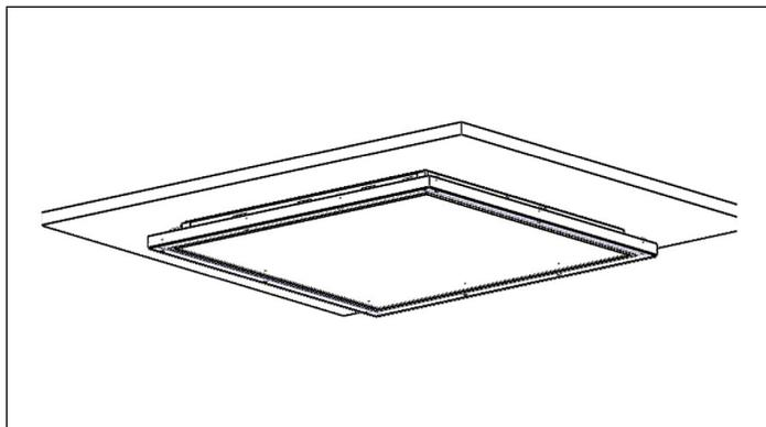
**STEP 7.** Remove protective film from the front surface of the light fixture when installation is completed.
