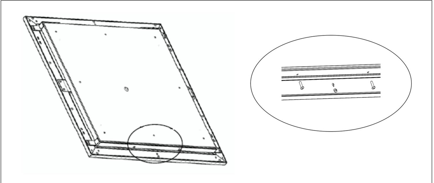
**STEP 11.** Secure luminaire to hangar bracket base using #8 ½" screws.
