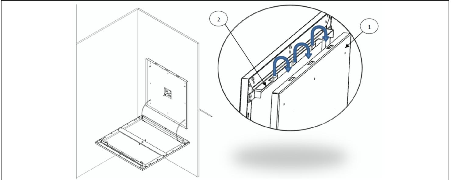
**STEP 9.** Reposition and attach safety cables to bottom of hanger bracket base and connect to luminaire. Secure the fixture to the **hanger bracket base [1]** by first inserting the tabs on the left side of the **hanger bracket [2]** into the slots of the **hanger bracket base [1]**.
