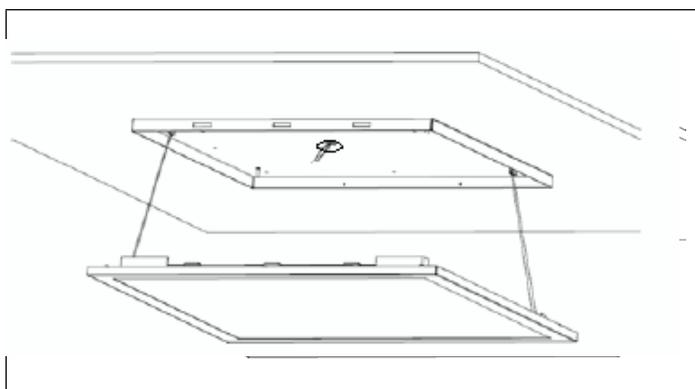
**STEP 3.** Attach safety cable from fixture to hanger bracket
