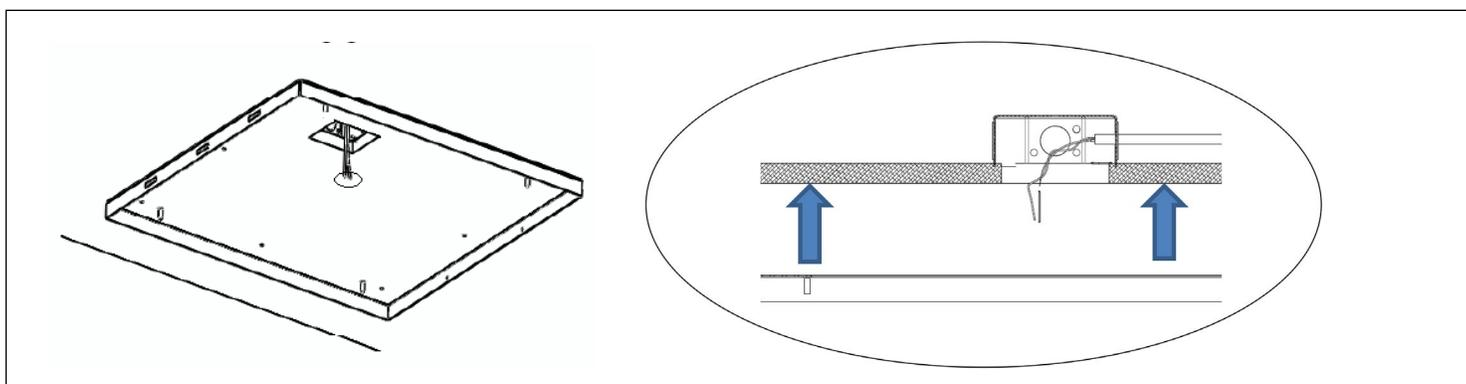
**STEP 2.** Install hanger bracket base (A) into ceiling.
