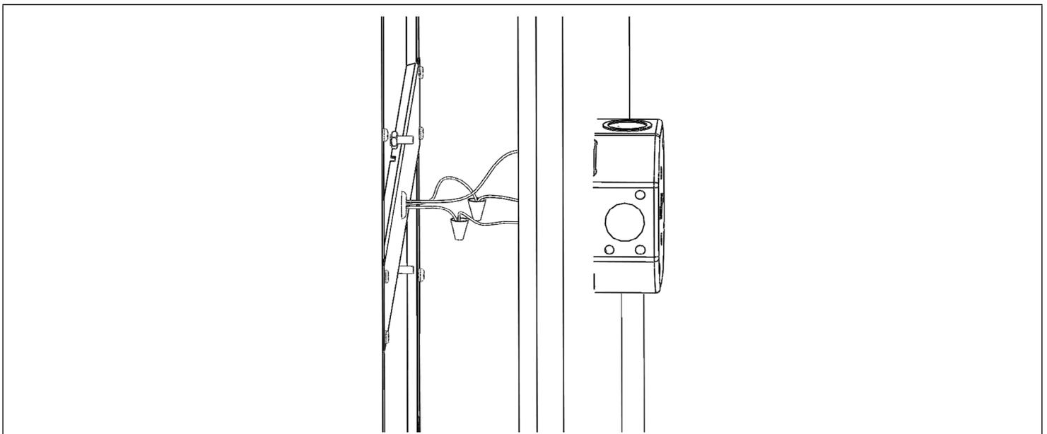
**STEP 10.** Wire fixture to remote driver. (Refer to wiring diagram from pg.2)
