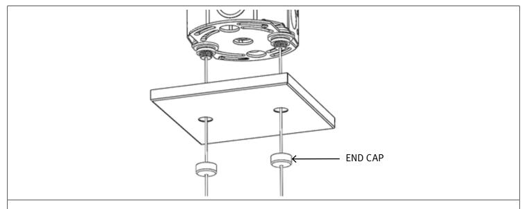
**STEP 6.** Raise canopy towards ceiling and attach to base plate using 4 end caps.
