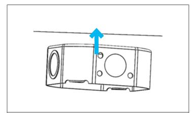
**STEP 2.** Secure Hex-Box (supplied by others) to a structure of suitable strength to support the fixture.
