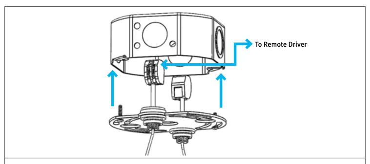
**STEP 5.** Remove end caps and lower canopy towards the fixture. Attach baseplate to the hex-box.
