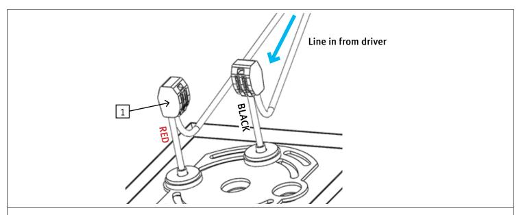
**STEP 3.** Connect black/red powered aircraft cable to line from the driver via the WAGO [1] or a similar electric connector. Refer to wiring diagram on page 2.
