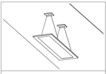
**7.** Remove protective film from the front surface of the light fixture when installation is completed.
