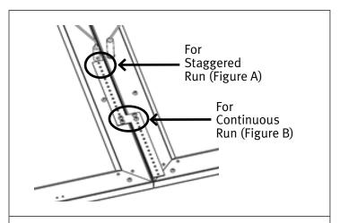
**8.** To create continuous chain, attach fixtures together using pendant connector bracket. Secure using screws.
