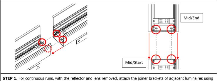
the two screws circled. Connect wires between luminaires as per the wiring diagram.
