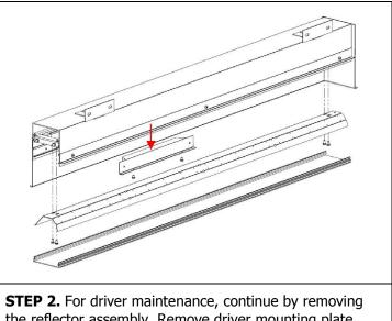
the reflector assembly. Remove driver mounting plate assembly, and service driver as required.
