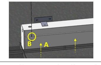
**STEP 4.** Lift luminaire up into ceiling and fasten to wall (A). Secure suspension cables to holes on fascia (B).
