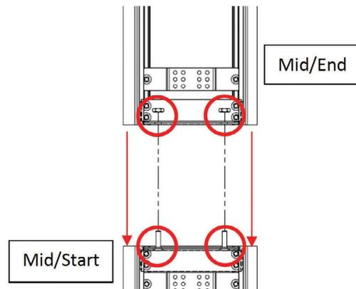
**STEP 6.** For continuous runs, with the reflector and lens removed, attach the joiner brackets of each unit using the two screws circled. Connect wires between luminaires as per the wiring diagram.
