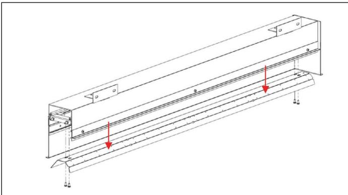
**STEP 3.** Unscrew fasteners to remove reflector assembly
