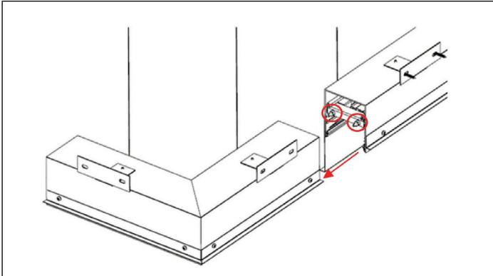
**STEP 7.** For corners, remove the lens and reflector pairs from the corner unit. Attach the corner to the preceding unit joiner bracket using the 2 screws shown. Connect wires between the luminaires as per the wiring diagram. Secure to ceiling as per step 5.
