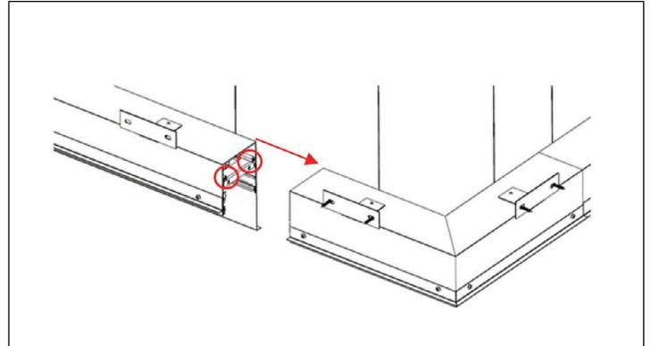
**STEP 8.** Attach the next mid/end unit to the corner unit as per step 6. Connect wires between luminaires as per the wiring diagram. Reinstall the reflector and lens in the corner.
