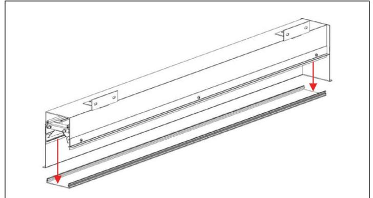
**STEP 2.** Remove the lens by gently pressing into the middle of the lens near the endcap and prying up the exposed edge.
