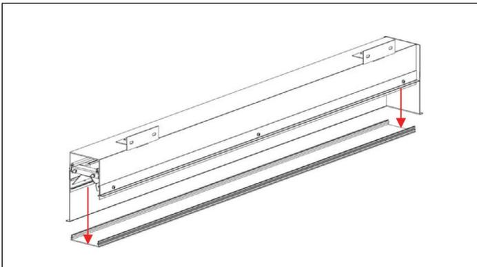
For LED board maintenance, remove the lens by gently pressing into the middle of the lens near the endcap and prying up the exposed edge.
