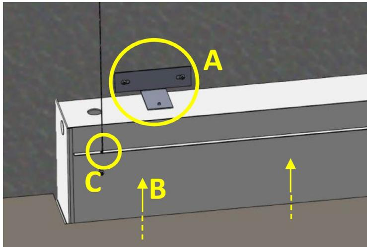
**STEP 5.** Install Wall Mounting Brackets above ceiling (A). Lift luminaire up into ceiling and reattach to Wall Mounting Bracket (B) by fastening them from the inside of the luminaire body. Secure suspension cables to holes on Fascia (C).
