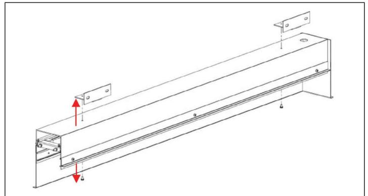
**STEP 4.** Unscrew fasteners from inside of Luminaire Body to free Wall Mounting Brackets.
